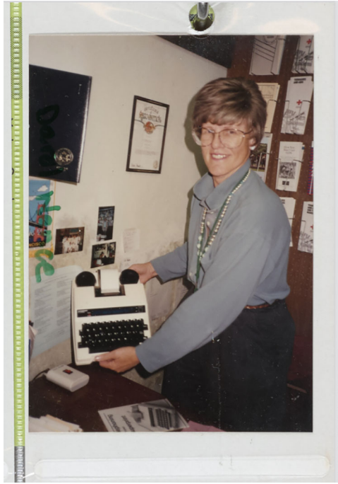
FIGURE 5. Nance shows off the Center's Telecommunications Device for the Deaf (TDD). A phone receiver was placed in the acoustic coupler on top of the teletypewriter (note the two black cradles designed to hold the receiver). When a user typed on the keyboard, acoustic tones corresponding to letters could be sent and received through a modem and telephone line. Scrapbook volume 1, 1987–1993, 2011, Deaf AIDS Center Collection (SFH 71), San Francisco History Center, San Francisco Public Library.
